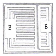
Top Material: Al Backside Material: Ag Bond Pad Size: .004" X .004" Backside Potential: Collector
